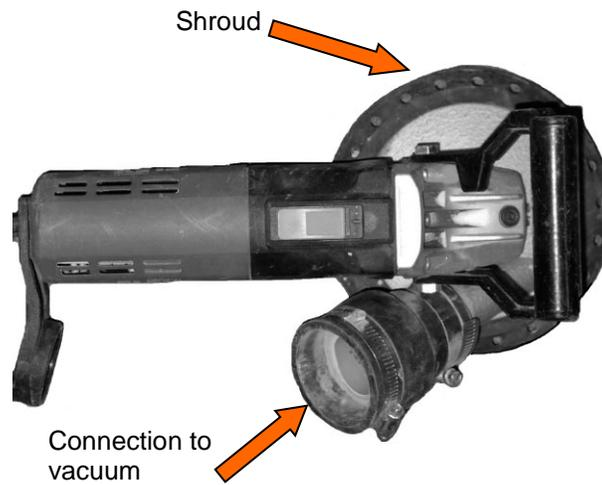
Figure 1 Hand held grinder, shroud and vacuum connection
